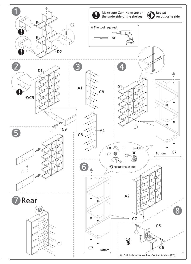
Please do not use excess force when inserting the Dowels. Using excess force can damage the panels during assembly.
