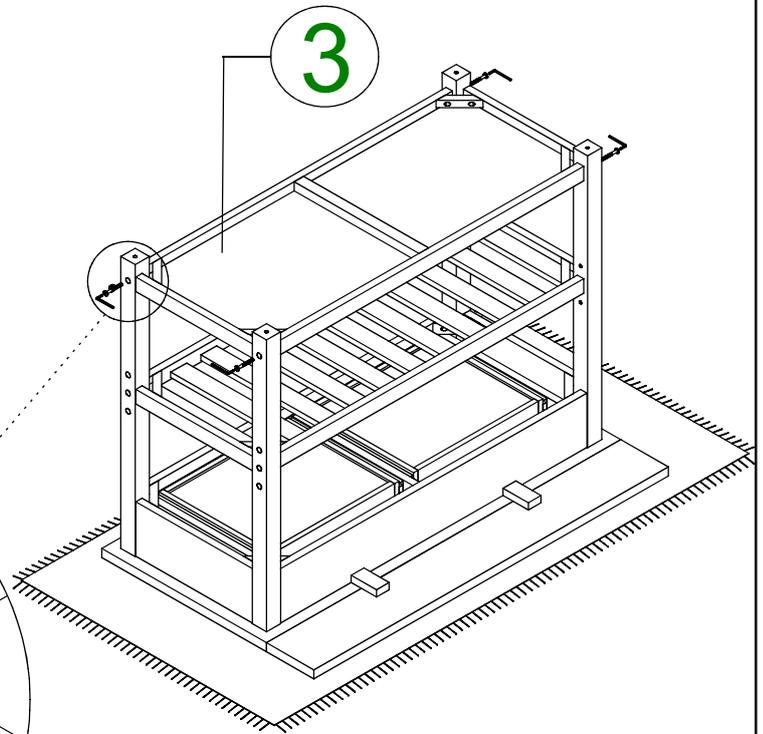
TIGHTEN BOLT COMPLETELY.
