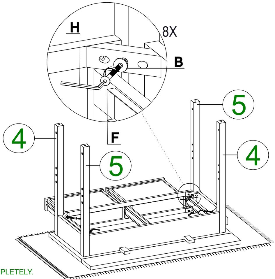
DO NOT TIGHTEN BOLT COMPLETELY.
