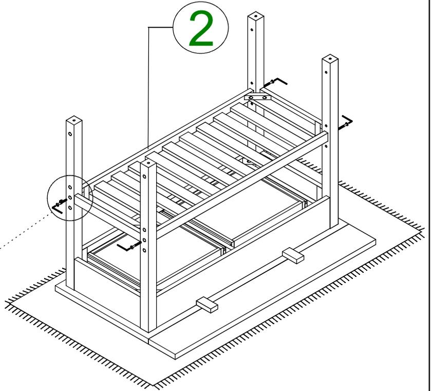
TIGHTEN BOLT COMPLETELY.
