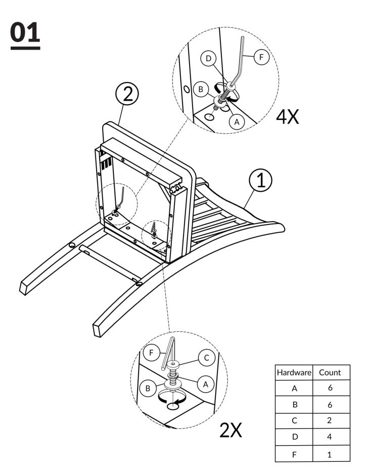
DO NOT TIGHTEN BOLT COMPLETELY.
