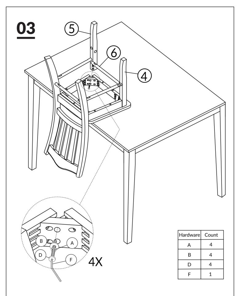
DO NOT TIGHTEN BOLT COMPLETELY.
