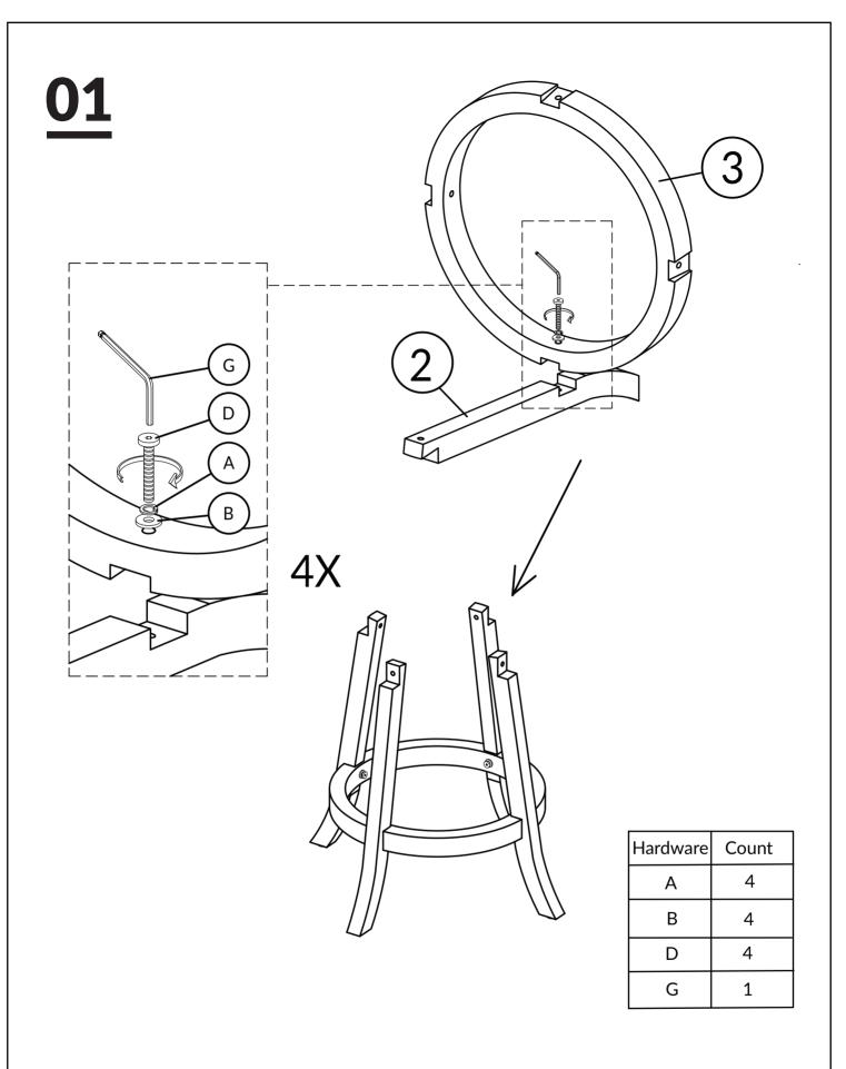
DO NOT TIGHTEN BOLT COMPLETELY.
