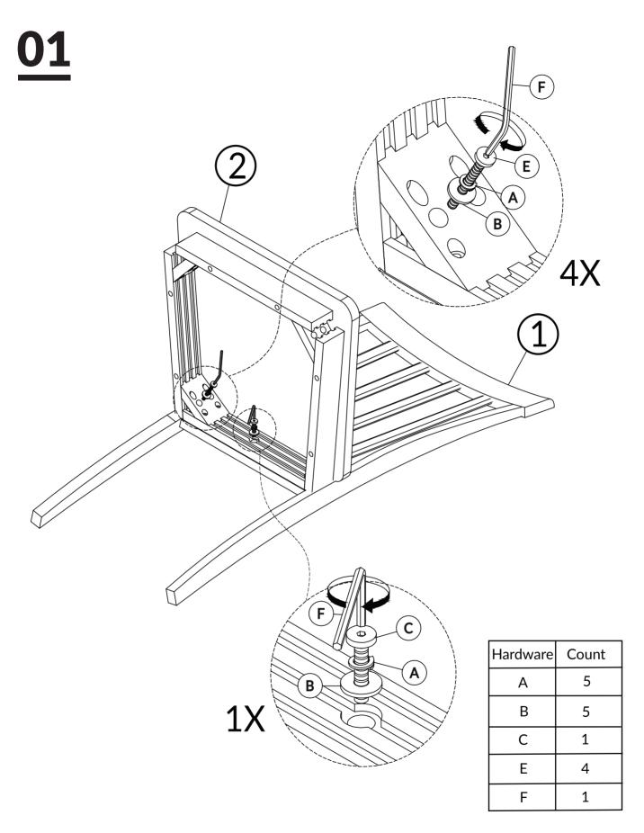
TIGHTEN BOLT COMPLETELY.
