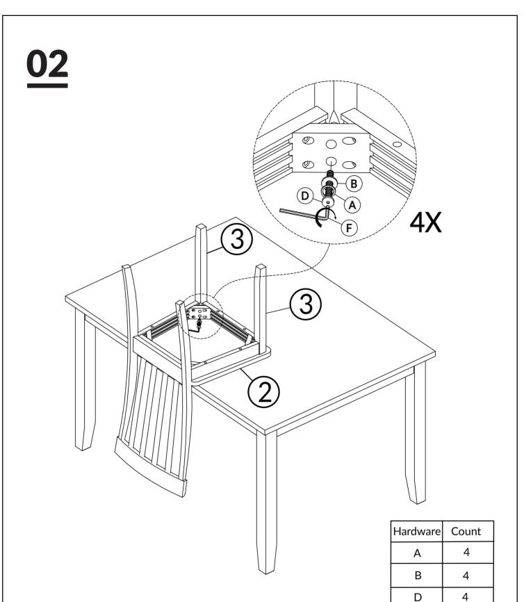
TIGHTEN BOLT COMPLETELY.
