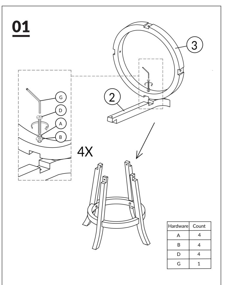
DO NOT TIGHTEN BOLT COMPLETELY.
