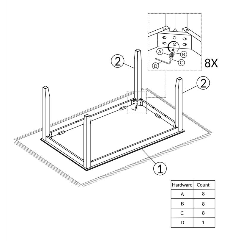
TIGHTEN BOLT COMPLETELY.
