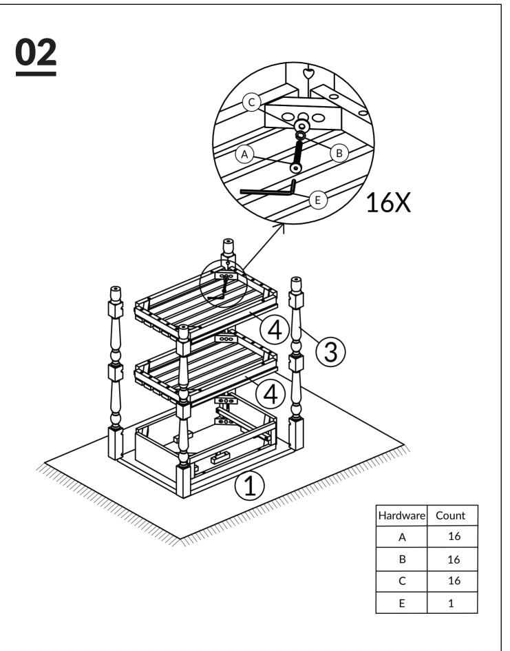
DO NOT TIGHTEN BOLT COMPLETELY.
