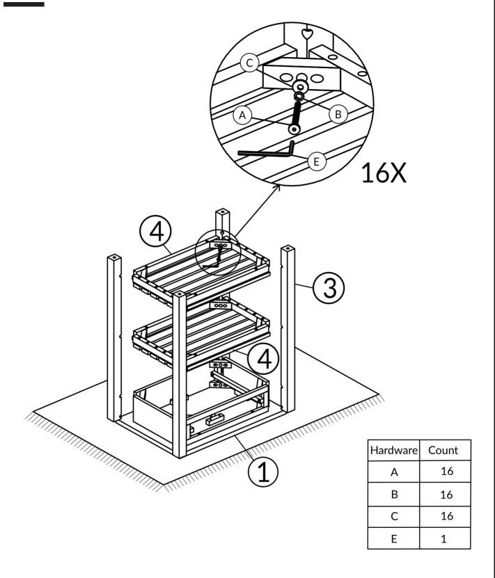
DO NOT TIGHTEN BOLT COMPLETELY.
