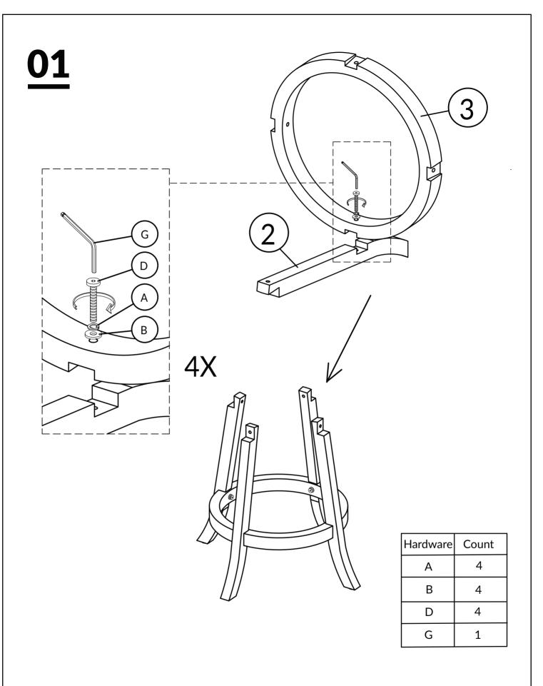
DO NOT TIGHTEN BOLT COMPLETELY.
