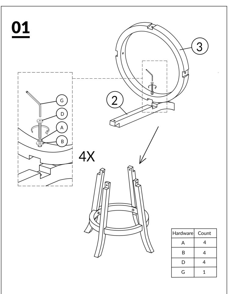
DO NOT TIGHTEN BOLT COMPLETELY.
