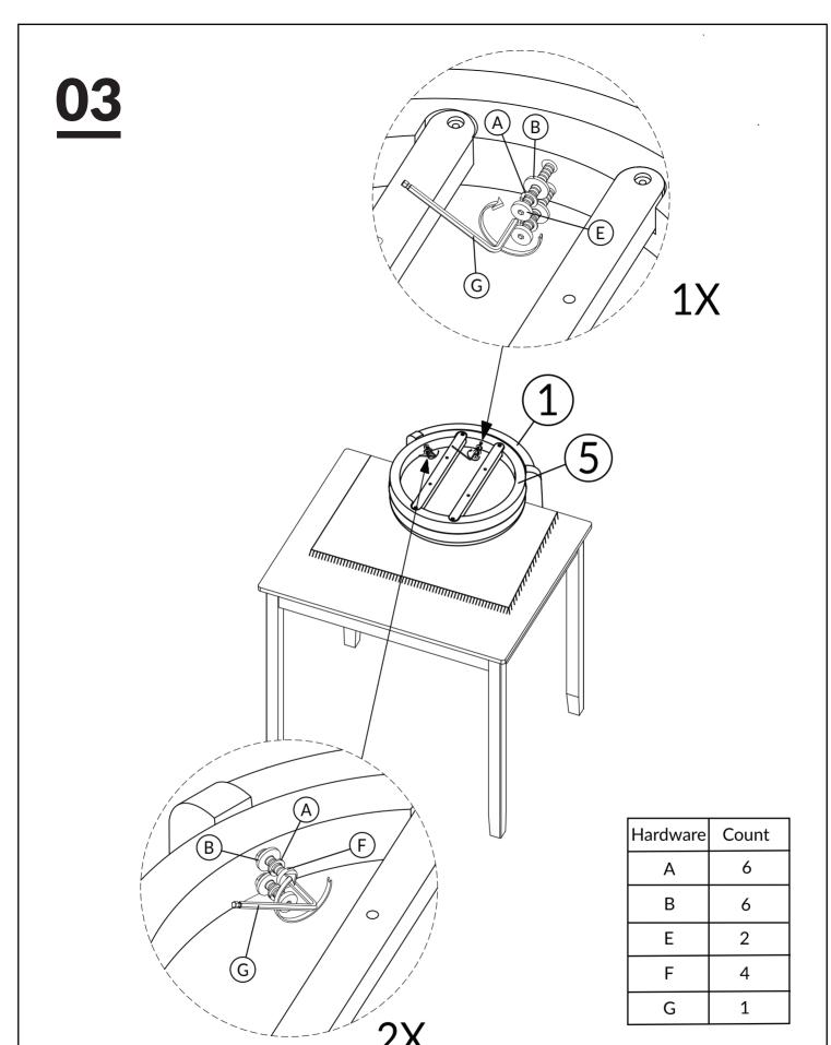
TIGHTEN BOLT COMPLETELY.
