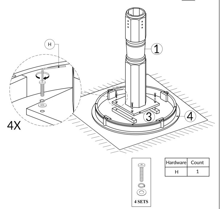
TIGHTEN BOLT COMPLETELY.
