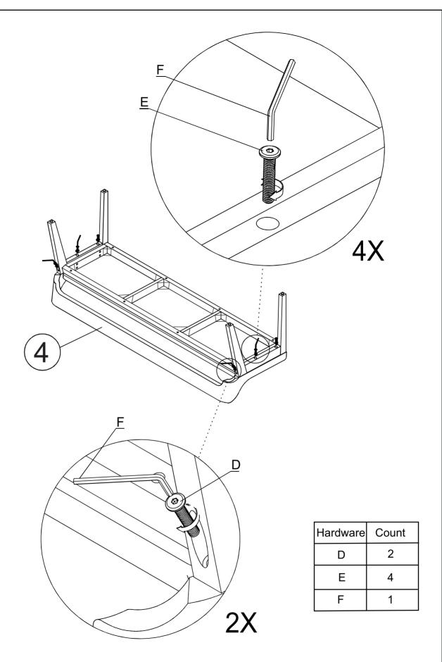
TIGHTEN BOLT COMPLETELY.
