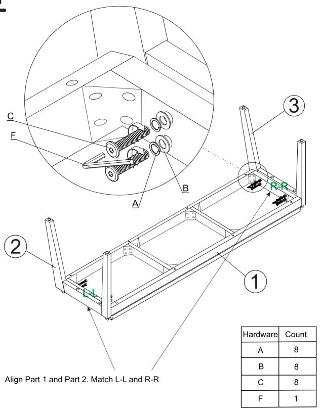
DO NOT TIGHTEN BOLT COMPLETELY.
