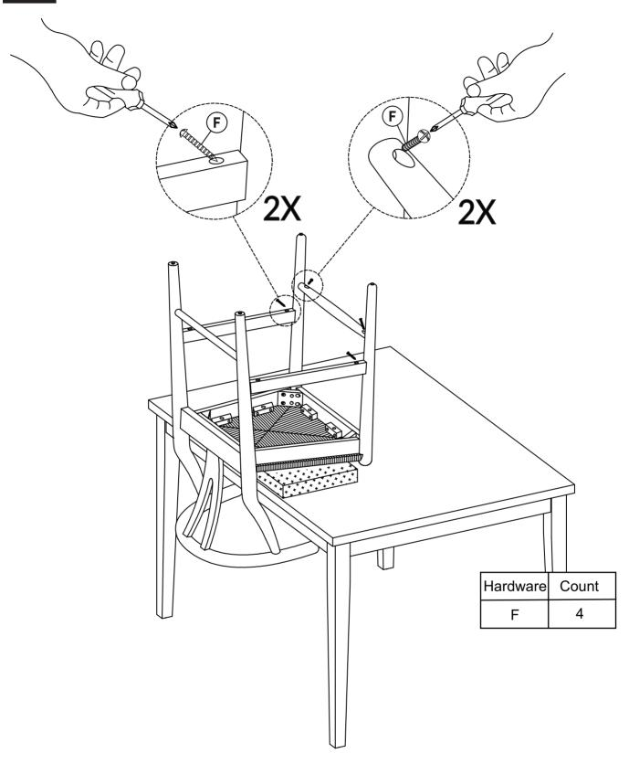
TIGHTEN BOLT AND SCREW COMPLETELY.
