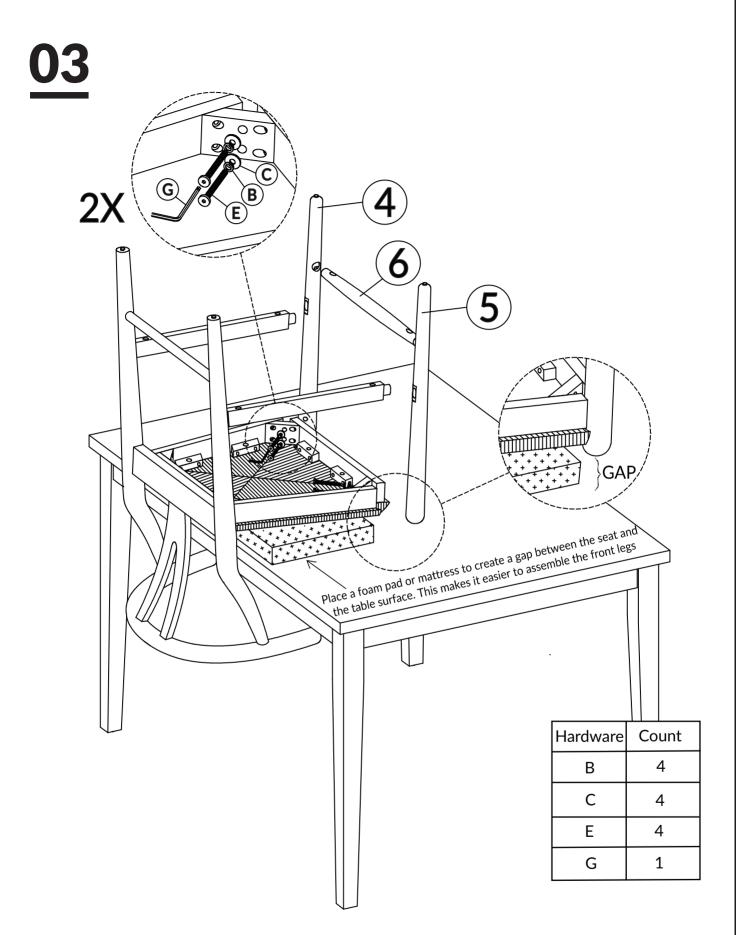
DO NOT TIGHTEN BOLT COMPLETELY.
