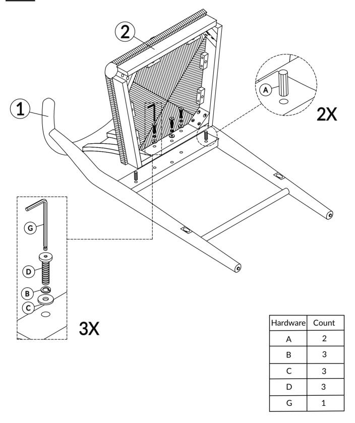
DO NOT TIGHTEN BOLT COMPLETELY.
