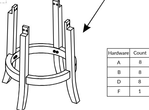
DO NOT TIGHTEN BOLT COMPLETELY.
