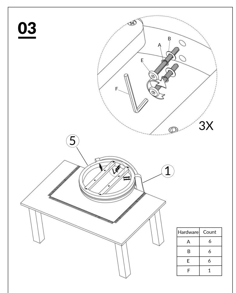
TIGHTEN BOLT COMPLETELY.
