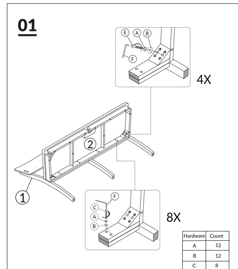
TIGHTEN BOLT COMPLETELY.
