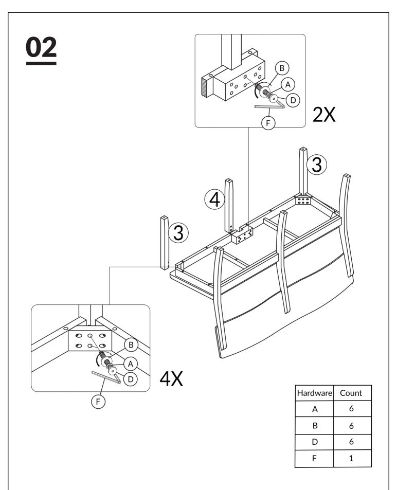
TIGHTEN BOLT COMPLETELY.
