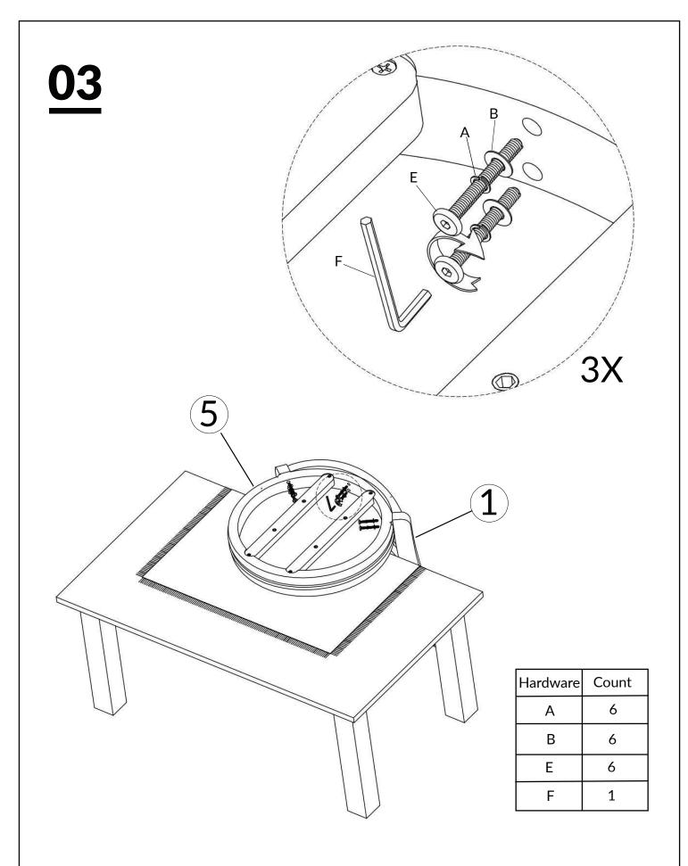
TIGHTEN BOLT COMPLETELY.
