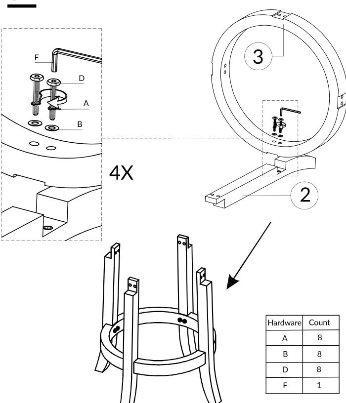
DO NOT TIGHTEN BOLT COMPLETELY.
