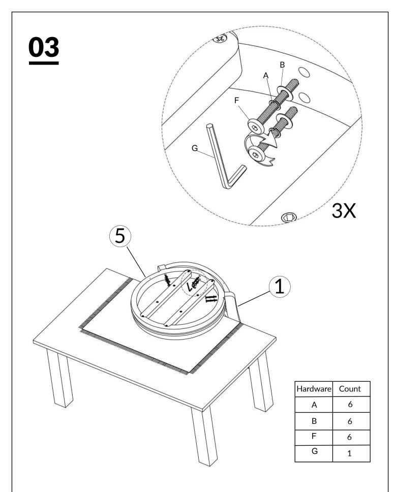
TIGHTEN BOLT COMPLETELY.
