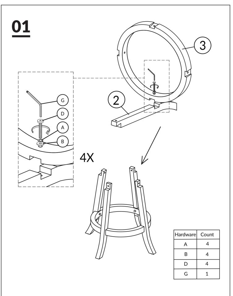
DO NOT TIGHTEN BOLT COMPLETELY.
