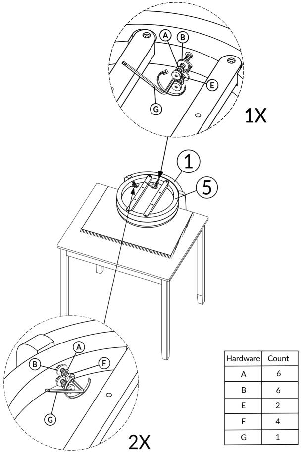
TIGHTEN BOLT COMPLETELY.
