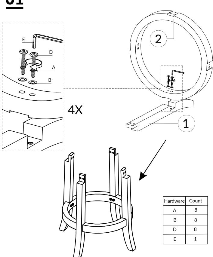
DO NOT TIGHTEN BOLT COMPLETELY.
