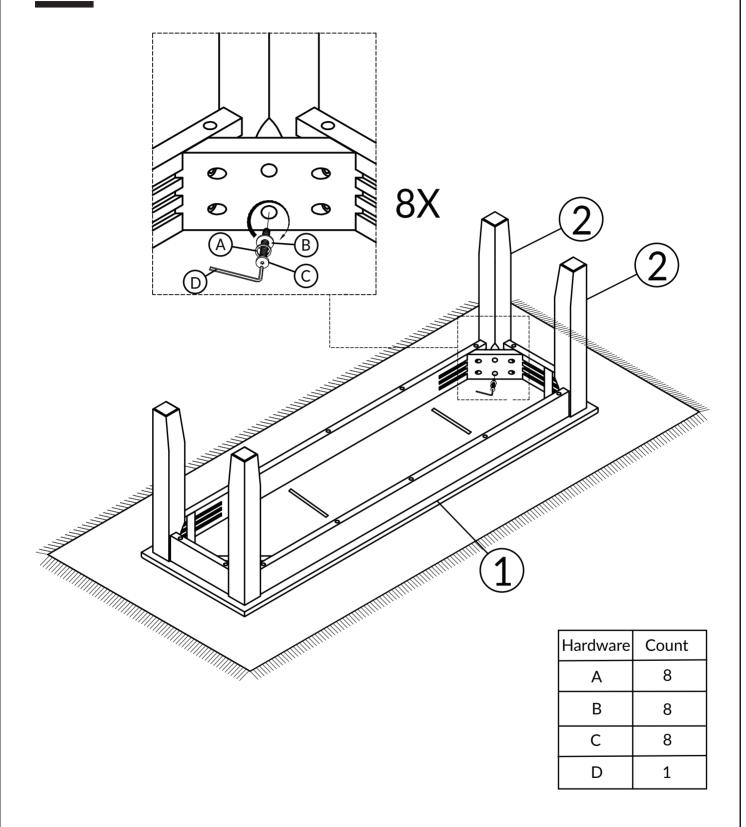
TIGHTEN BOLT COMPLETELY.
