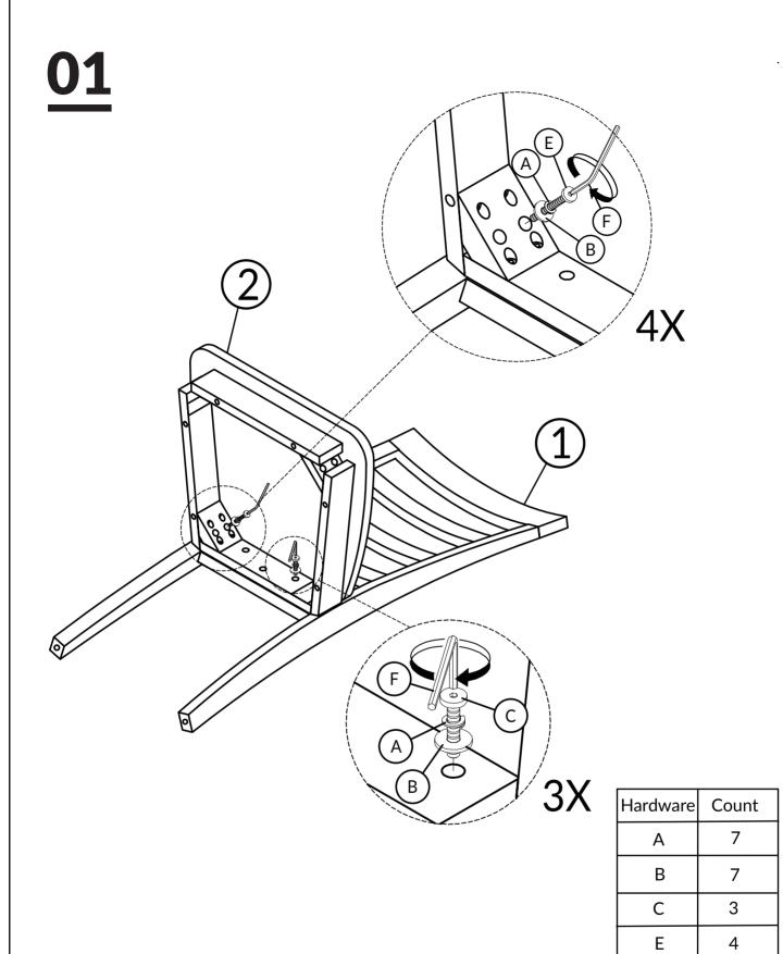
TIGHTEN BOLT COMPLETELY.
