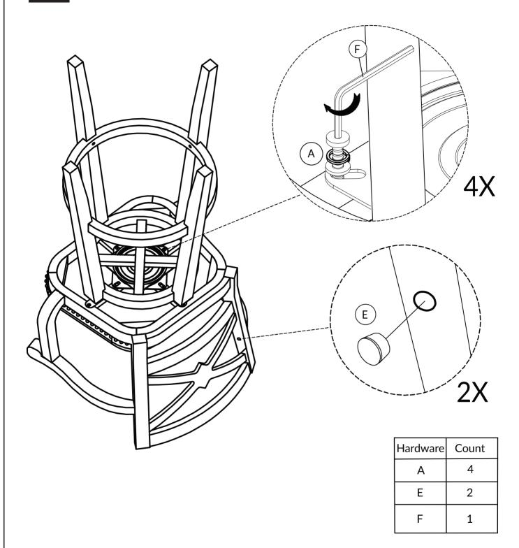
TIGHTEN BOLT COMPLETELY.
