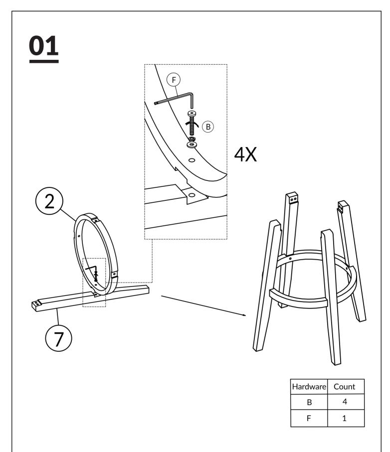
DO NOT TIGHTEN BOLT COMPLETELY.
