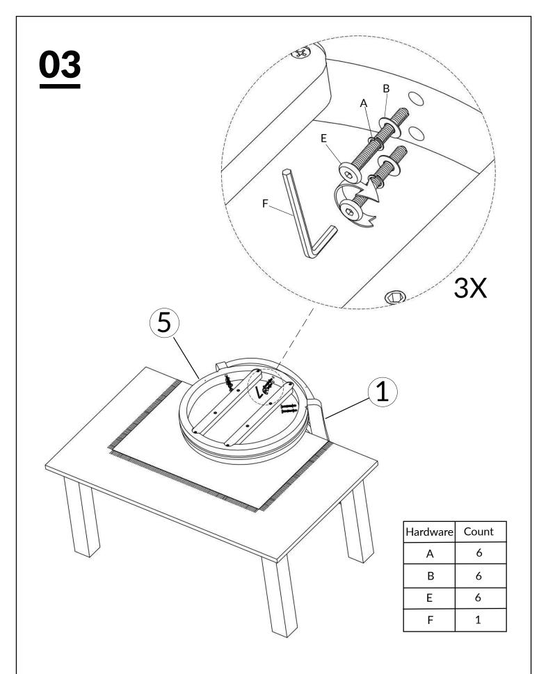
TIGHTEN BOLT COMPLETELY.
