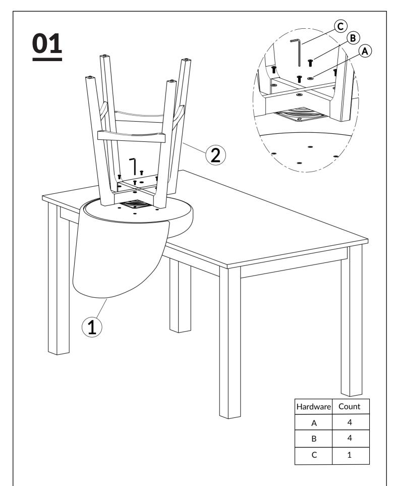
TIGHTEN BOLT COMPLETELY.
