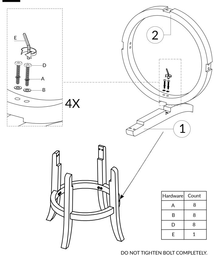
Please make sure that the protective metal kick plate from Footrest (Part #2) is facing upwards. Remove the white Tape from the protective metal kick plate before using.
