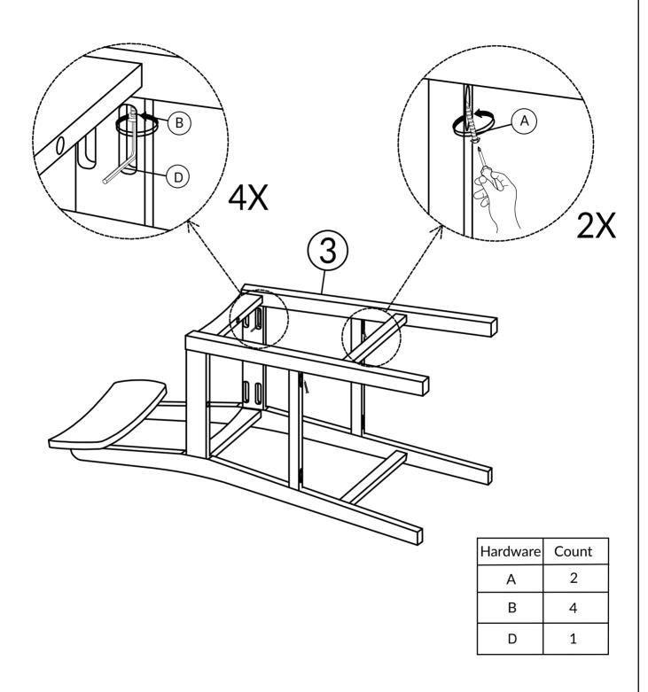
DO NOT TIGHTEN BOLT AND SCREW COMPLETELY.
