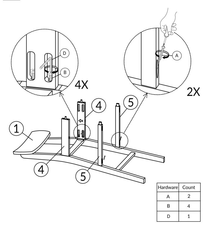
Attach part 4 by following the arrow direction shown in the picture above to ensure correct alignment.
