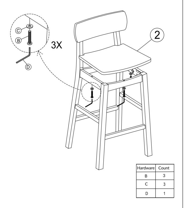
TIGHTEN BOLT AND SCREW COMPLETELY.
