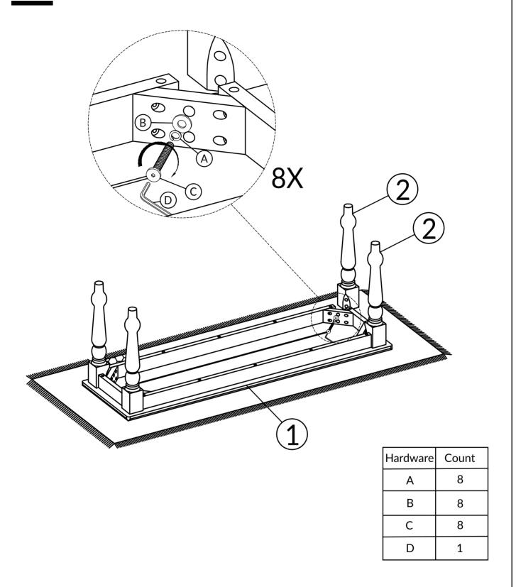
TIGHTEN BOLT COMPLETELY.
