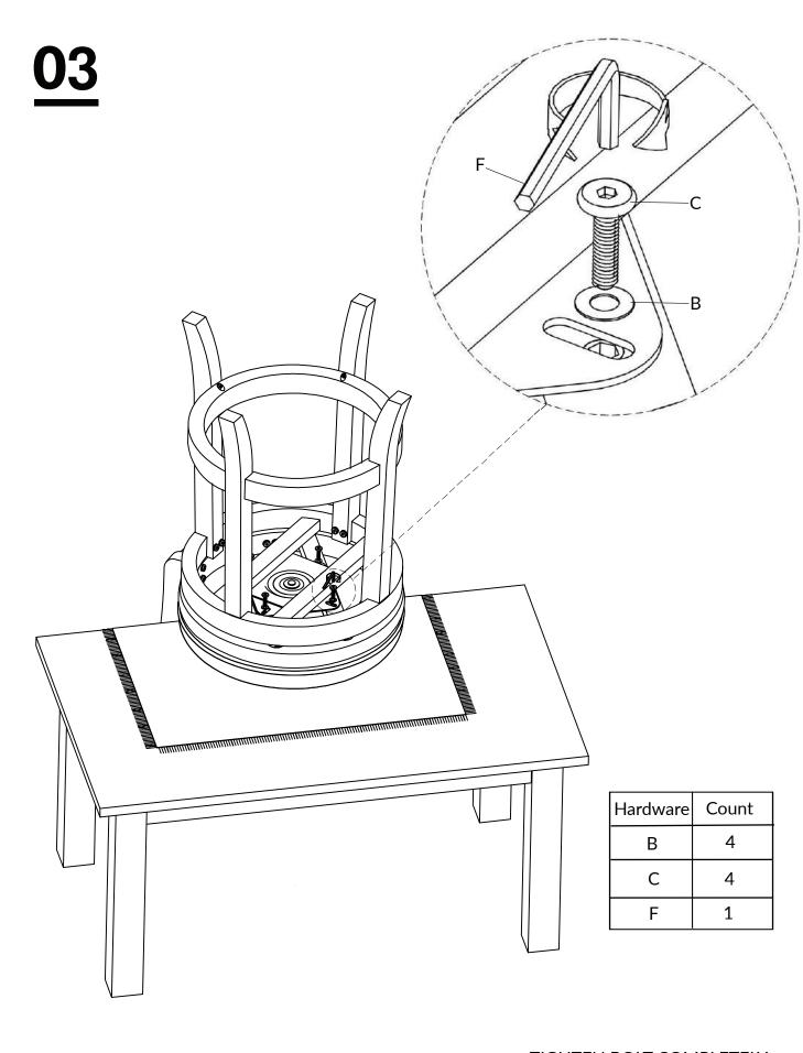
TIGHTEN BOLT COMPLETELY.
