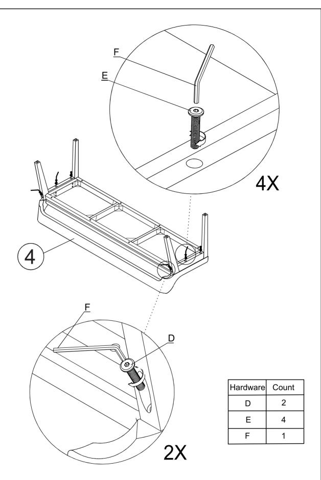
TIGHTEN BOLT COMPLETELY.
