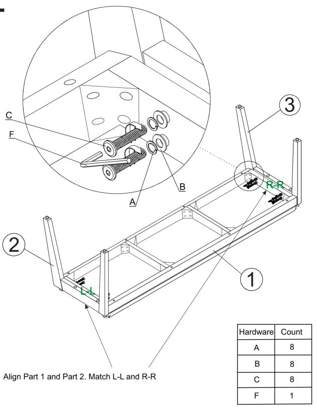
DO NOT TIGHTEN BOLT COMPLETELY.
