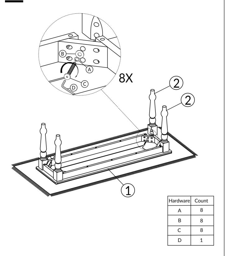
TIGHTEN BOLT COMPLETELY.
