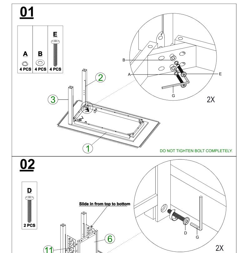
DO NOT TIGHTEN BOLT COMPLETELY.
