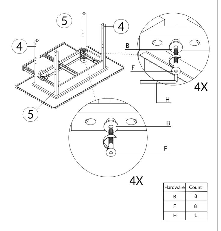
DO NOT TIGHTEN BOLT COMPLETELY.
