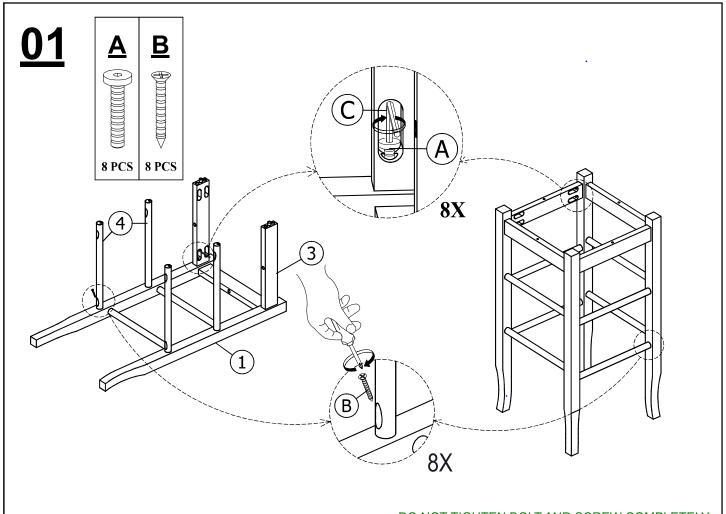
DO NOT TIGHTEN BOLT AND SCREW COMPLETELY.
