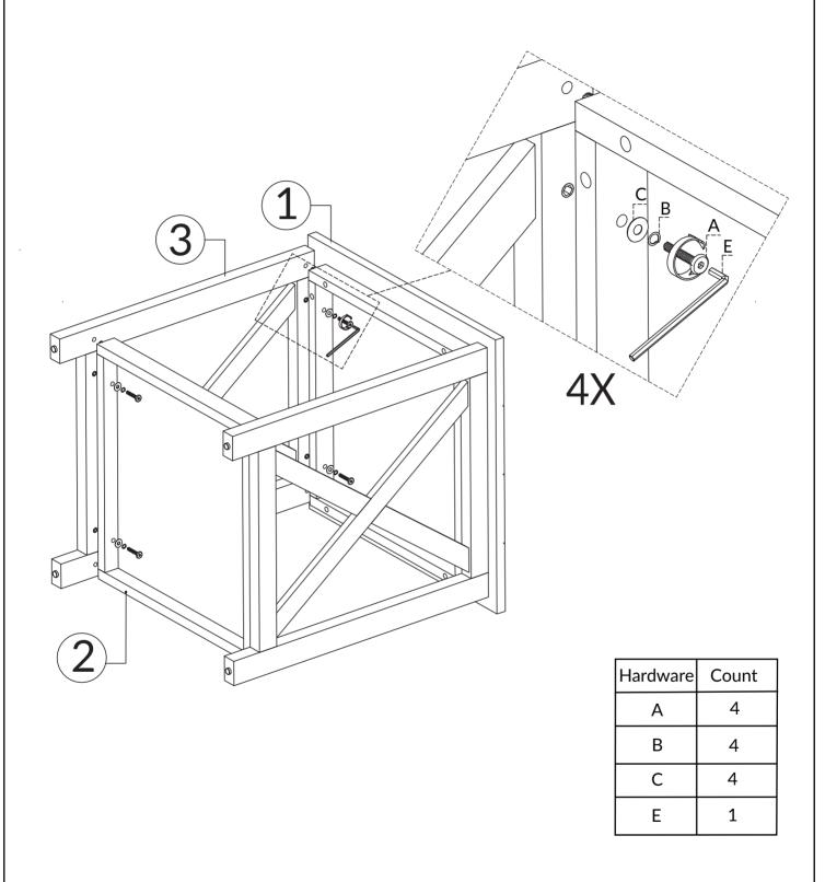
TIGHTEN BOLT COMPLETELY.
