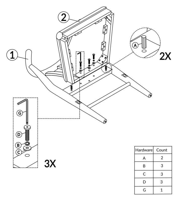
DO NOT TIGHTEN BOLT COMPLETELY.
