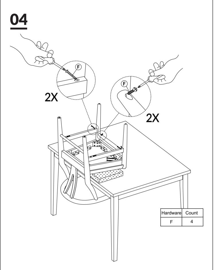
TIGHTEN BOLT AND SCREW COMPLETELY.
