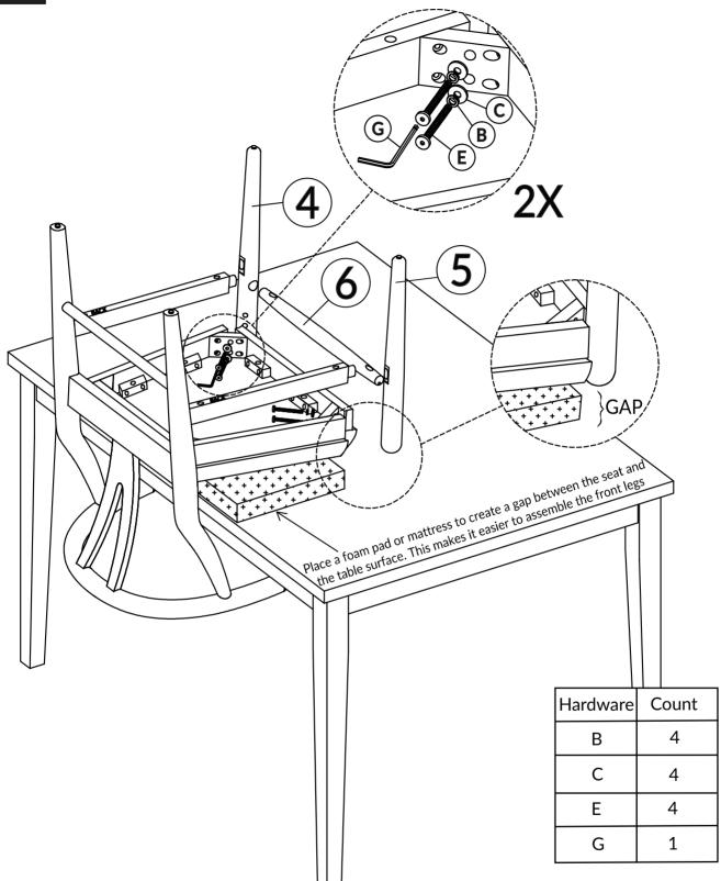
DO NOT TIGHTEN BOLT COMPLETELY.
