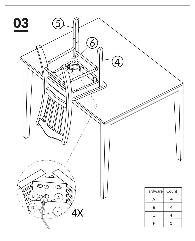
DO NOT TIGHTEN BOLT COMPLETELY.
