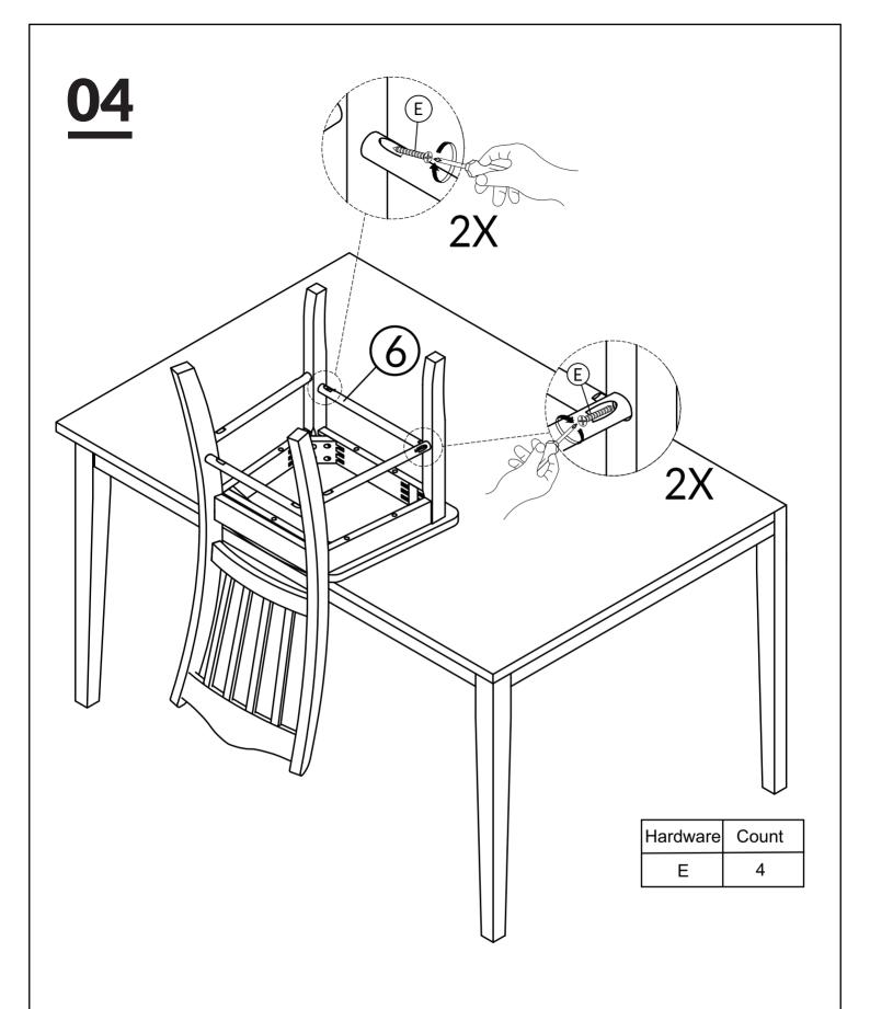
TIGHTEN BOLT AND SCREW COMPLETELY.
