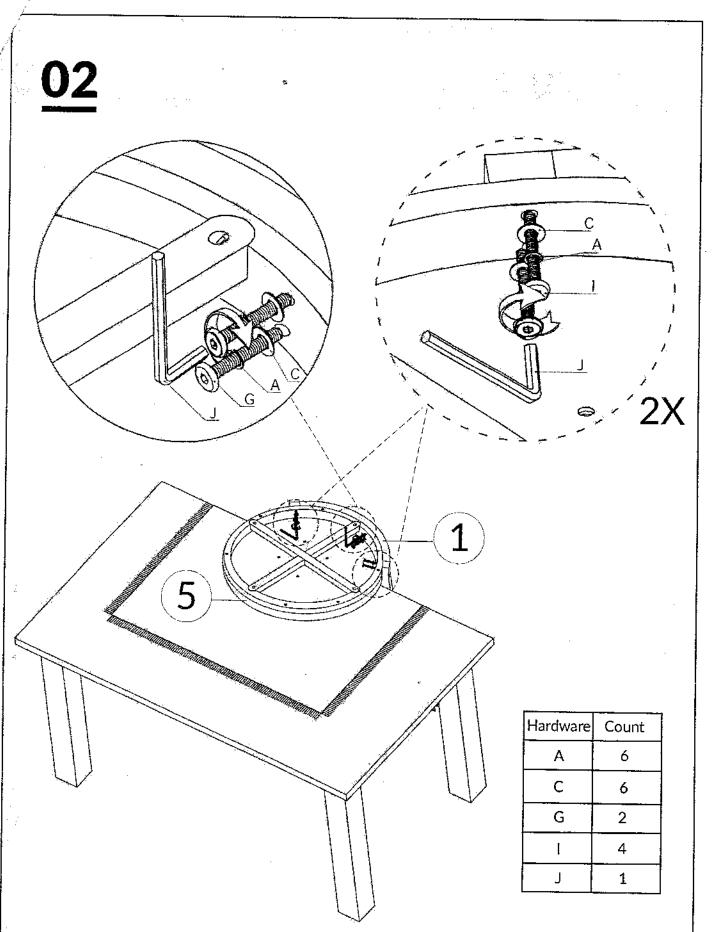
TIGHTEN BOLT COMPLETELY.
