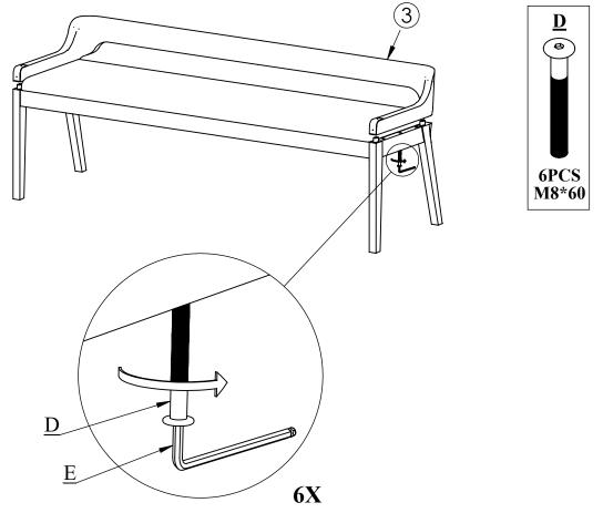
DO NOT TIGHTEN BOLT COMPLETELY
