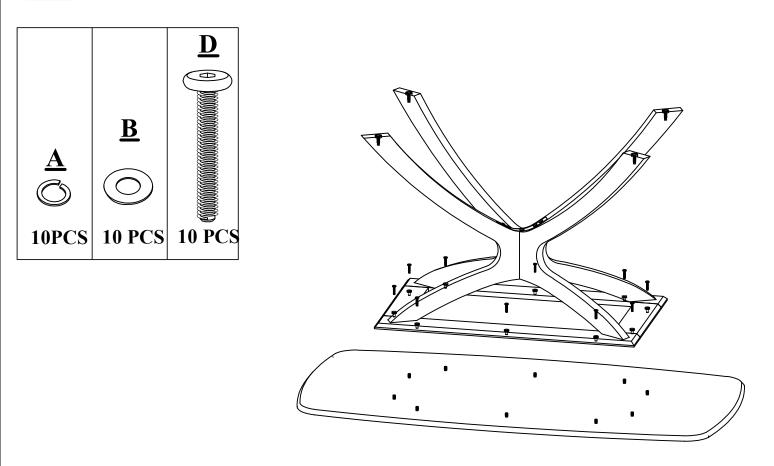
DO NOT TIGHTEN BOLT COMPLETELY.
