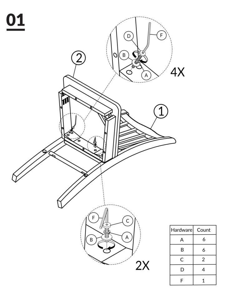
DO NOT TIGHTEN BOLT COMPLETELY.
