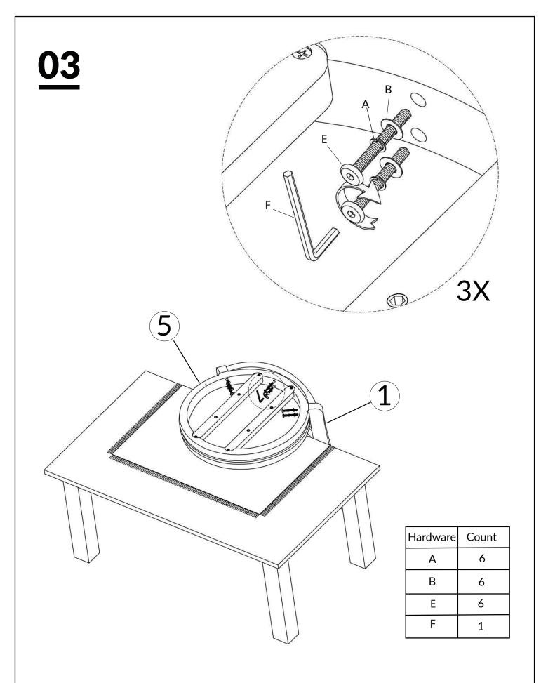
TIGHTEN BOLT COMPLETELY.
