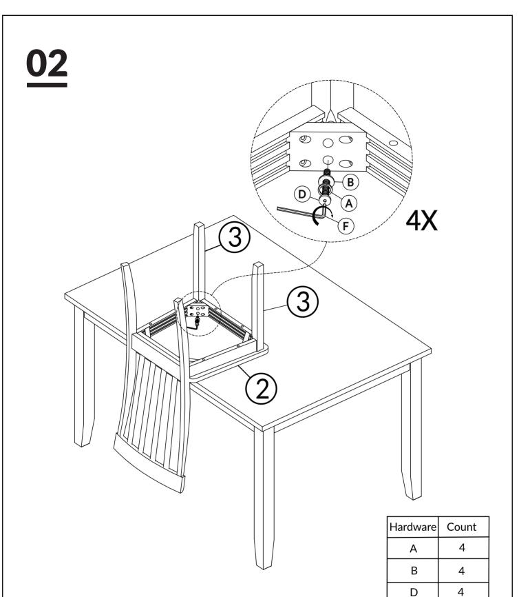
TIGHTEN BOLT COMPLETELY.
