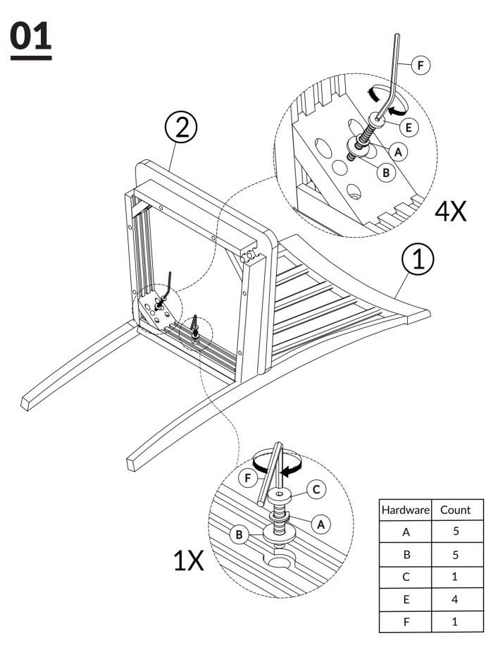
TIGHTEN BOLT COMPLETELY.
