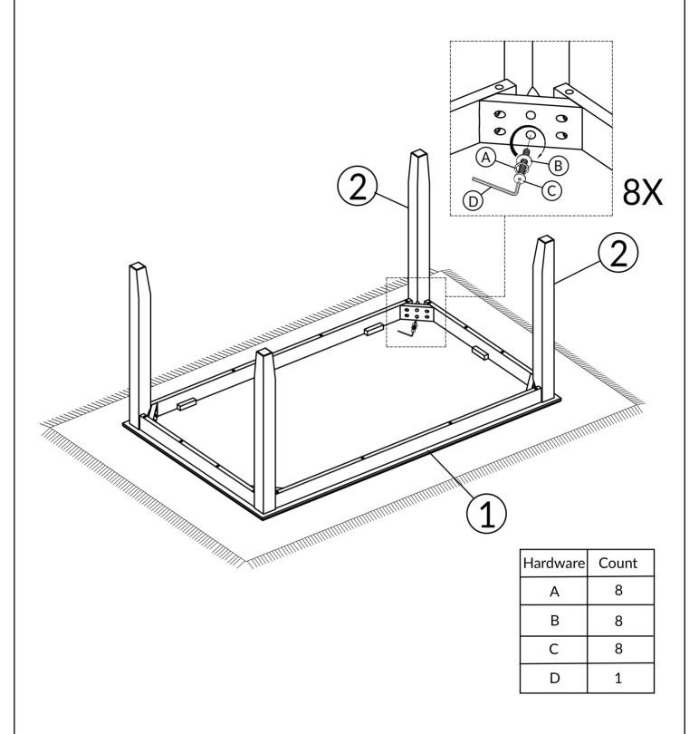
TIGHTEN BOLT COMPLETELY.
