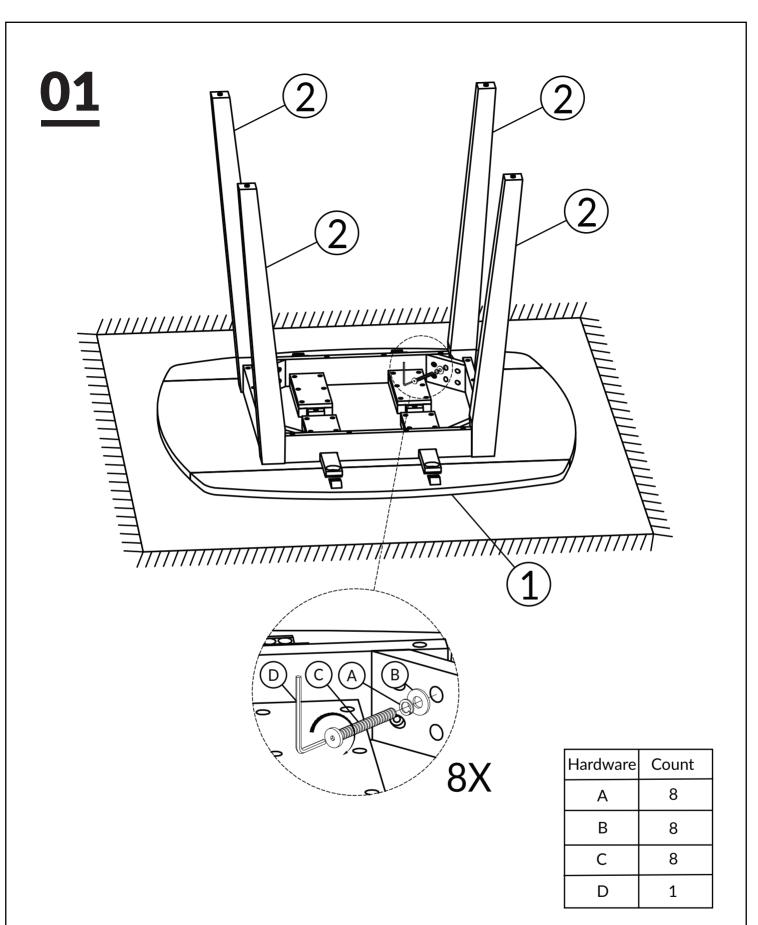
TIGHTEN BOLT COMPLETELY.
