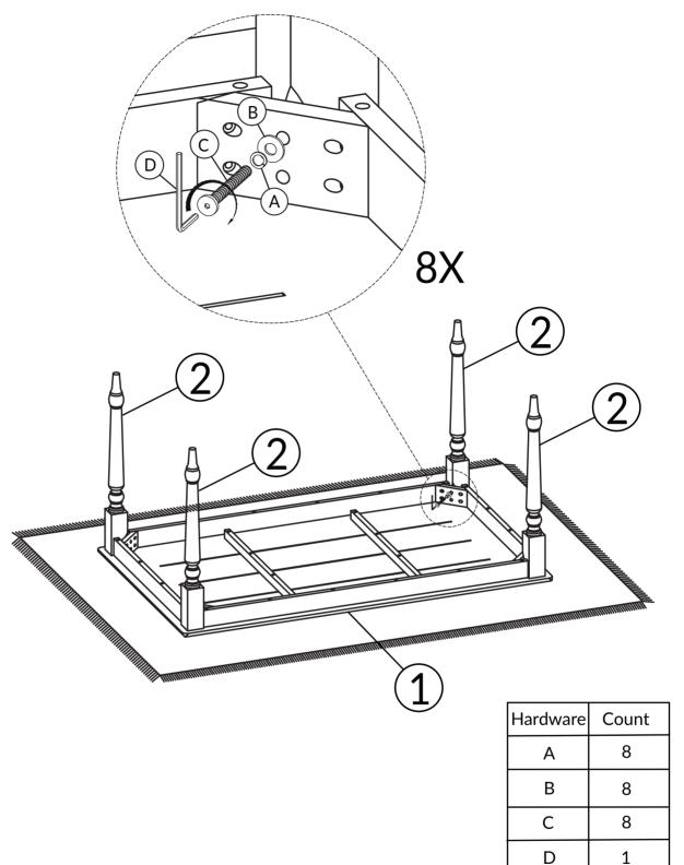
TIGHTEN BOLT COMPLETELY.
