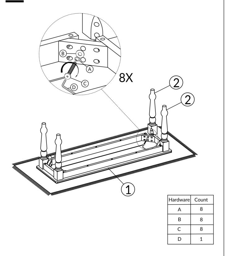
TIGHTEN BOLT COMPLETELY.
